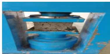
Fig (u): Compression test of concrete cubes
