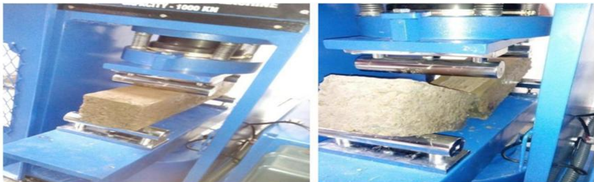
Fig (q): Flexure strength testing of beam moulds
