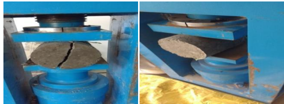
Fig(p): Testing of cylinder moulds
