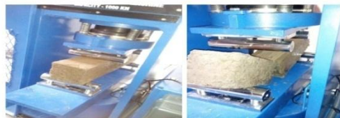
Fig (w): Flexure strength test of beam moulds
