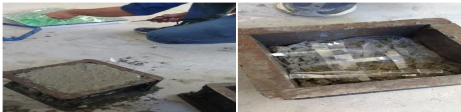
Fig (n): Casting of cube moulds with thread shaped plastic bottles
